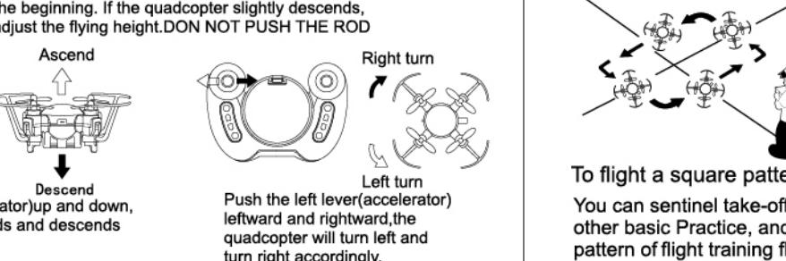
Push the left lever(accelerator) up and down, the quadcopter will ascends and descends accordingly.
